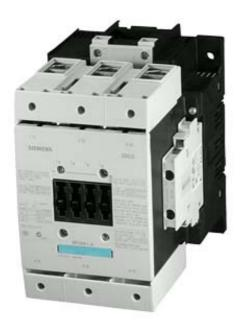
CONTACTOR, 55KW/400V/AC-3 AC(40...60HZ)/DC OPERATION UC 200...220V AUXIL. CONTACTS 2NO+2NC 3-POLE, SIZE S6 WITH BOX TERMINALS CONVENTIONAL OPERATING MECHAN. SCREW TERMINAL
