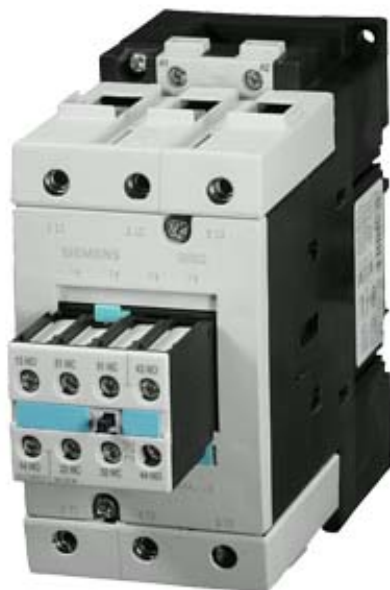
CONTACTOR, AC-3 45 KW/400 V, AC 24V 50/60HZ, 2 NO + 2 NC, 3-POLE, SIZE S3, SCREW CONNECTION
