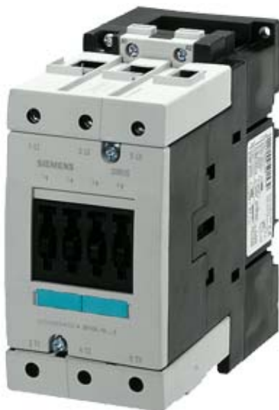
CONTACTOR, AC-3 45 KW/400 V, AC 24V 50/60HZ 3-POLE, SIZE S3, SCREW CONNECTION
