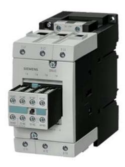
CONTACTOR, AC-3 37 KW/400 V, DC 110 V, 2 NO + 2 NC, 3-POLE, SIZE S3, SCREW CONNECTION
