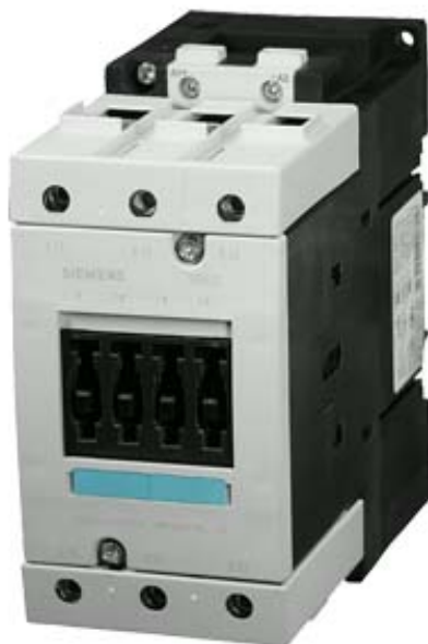
CONTACTOR, AC-3 37 KW/400 V, DC 42 V, 3-POLE, SIZE S3, SCREW CONNECTION
