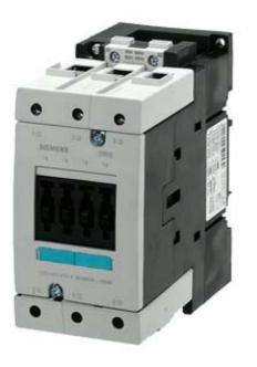
CONTACTOR, AC-3 37 KW/400 V, AC 230 V, 50 HZ, 3-POLE, SIZE S3, SCREW CONNECTION MOUNTING POSITION VERTICAL
