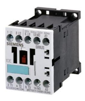
CONTACTOR, AC-3 3 KW/400 V, 1 NO, AC 24 V, 50/60 HZ, 3-POLE, SIZE S00, SCREW CONNECTION, MOUNTING POSITION VERTICAL
