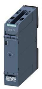
TIME RELAY, ELECTRONIC, WITH STAR-DELTA FUNCTION, 1 CONTACTOR DELAYED, 1 CONTACTOR NON-DELAYED, 1 TIME SET. RANGE 1...20S, 12V...240V AC/DC AT AC 50/60HZ, SCREW TERMINAL
