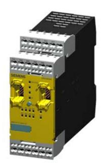
SIRIUS, CENTRAL MOD. 3RK3 BASIC FOR MODULAR SAFETY SYSTEM 3RK3 4/8 F-DI, 1 F-RO, 1 F-DO, 24V DC PARAMETERIZABLE VIA SW MSS ES 45MM WIDE SPRING-LOADED TERMINAL UP TO SIL3 (IEC 61508) UP TO PERFORMANCE LEVEL E (ISO 13849-1)
