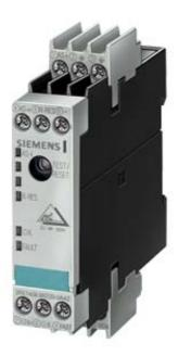
AS-INTERFACE SLIMLINE MODULE S22.5, EARTH FAULT MONITORING, IP20,1 X 1INPUT, REMOTE RESET, 2 X SIGNAL OUTPUT, RELAY, 1A DC12 1A (2A MAX.) DC13 500MA (24V) SCREW-TYPE TERMINAL CONNECT., MODULE WIDTH 22.5 MM, NO AS-I ADDRESS REQUIRED AS-INTERFACE MONITORING ONLY
