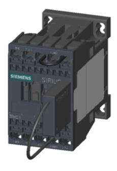
CONTACTOR RELAY FOR RAILWAY, 2NO+1NC, DC 125V, 0.7..1.25\*US, W/ INTEGRATED SUPPRESSOR DIODE, SIZE S00, SCREW TERMINAL, OPTIMIZED MOUNTING (20G)
