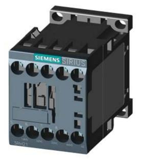
CONTACTOR RELAY, 2NO+2NC, AC 230V, 50/60 HZ, SIZE S00, SCREW TERMINAL, OPTIMIZED MOUNTING (20G)
