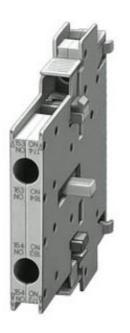
AUX. SWITCH BLOCK, 1NO+1NC, DIN EN50005, LATERALLY, 10 MM SCREW CONNECTION, SIZE S0...S12, FOR CONTACTORS FOR SWITCHING MOTORS, 2-POLE
