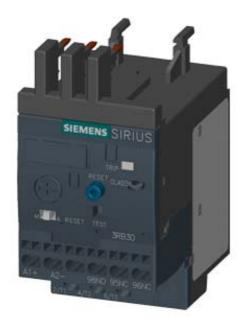
OVERLOAD RELAY 0.32...1.25 A FOR MOTOR PROTECTION SIZE S00, CLASS 10 CONTACTOR ASS. MAIN CIRCUIT: SPR.-LOAD.TERM. AUX.CIRCUIT: SPR.-LOAD.TERM. MANUAL-AUTOM.-RESET
