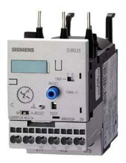
OVERLOAD RELAY 0.1...0.4 A FOR MOTOR PROTECTION SZ S0, CLASS 20 F. MOUNTING ONTO CONTACTORS MAIN CIRCUIT: SCREW TERMINAL AUX. CIRCUIT: SPRING-LOADED TERM. MANUAL-AUTOMATIC-RESET
