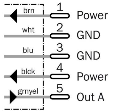
Connection diagram, Encoder connection
