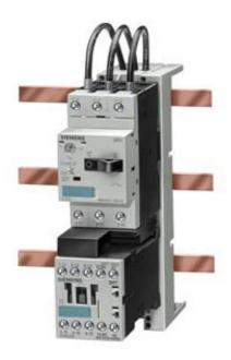
LOAD FEEDER FUSELESS DIRECT STARTING,AC 400V,SIZES00 0.35...0.5 A, AC 110 V, 50 HZ, 1NO(CONTACTOR), SCREW CONNECT. ON 40 MM BUSBAR ADAPTER TYPE OF COORDIN. 2, IQ = 50 KA
