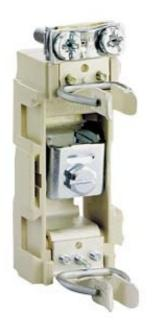
LV HRC BUS MOUNTING FUSE BASE 660V, 1-POLE, 160A, SIZE 00 FOR MOUNTING ONTO BUSBARS TERMINAL **CLAMP AT BOTTOM**
