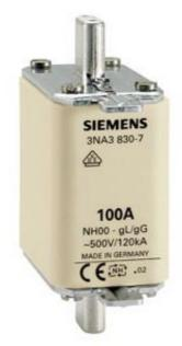
LV HRC FUSE LINK GL/GG WITH NON-INSULATED GRIP LUGS WITH FRONT INDICATOR SIZE 00, 125A, AC 500V/DC 250V
