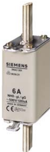
LV HRC FUSE LINK GL/GG WITH NON-INSULATED GRIP LUGS WITH FRONT INDICATOR SIZE 0, 6A, AC 500V/DC 440V
