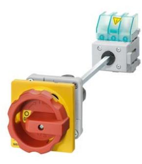
EMERG. STOP SWITCH 4-POLE IU=32, P/AC-23A AT 400V=11.5KW FLOOR MOUNTING DIN RAIL/TWO-HOLE MOUNTING ROTARY ACTUATOR RED/YELLOW (EMERG. STOP)
