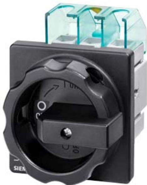
MAIN CONTROL SWITCH 3-POLE IU=32, P/AC-23A AT 400V=11,5KW FRONT MOUNTING FOUR- HOLE MOUNTING ROTARY ACTUATOR BLACK
