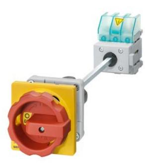
EMERG. STOP SWITCH 4-POLE IU=16, P/AC-23A AT 400V=7.5KW FLOOR MOUNTING DIN RAIL/TWO-HOLE MOUNTING ROTARY ACTUATOR RED/YELLOW (EMERG. STOP) FOUR-HOLE MOUNTING
