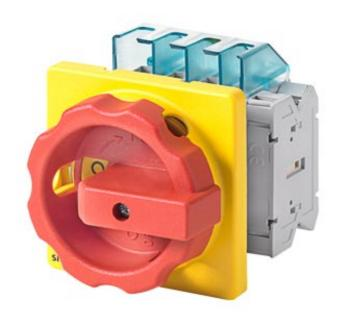
EMERG. STOP SWITCH 3-POLE IU=16, P/AC-23A AT 400V=7.5KW 1NO+1NC, FRONT MOUNTING FOUR-HOLE MOUNTING ROTARY ACTUATOR RED/YELLOW (EMERG. STOP)
