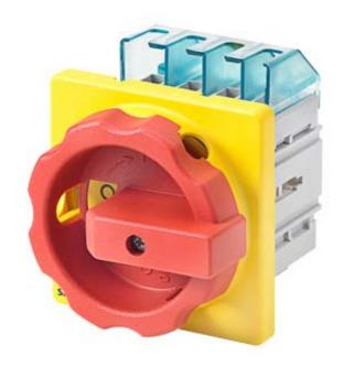
EMERG. STOP SWITCH 4-POLE IU=16, P/AC-23A AT 400V=7.5KW FRONT MOUNTING FOUR-HOLE MOUNTING ROTARY ACTUATOR RED/YELLOW (EMERG. STOP)
