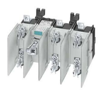
SWITCH DISCONNECTOR FUSE NEW DESIGN IU=63A, UE=690V, 3-POLE FOR LV HRC FUSE SIZE 00 BASIC VERSION WITHOUT 8UC6 HANDLE AND SHAFT
