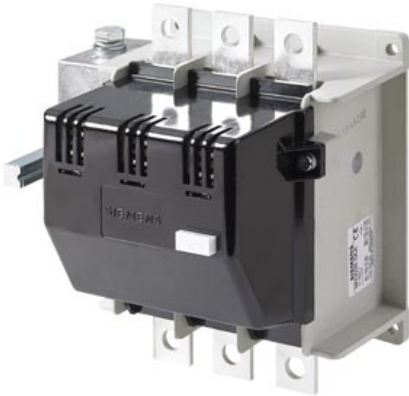
SWITCH DISCONNECTOR 3-POLE I=630A, U=690V, FRONT ROTARY OPERATING MECHANISM WITHOUT HANDLE
