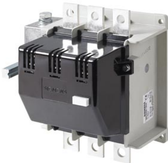
SWITCH DISCONNECTOR 3-POLE I=400A, U=690V, FRONT ROTARY OPERATING MECHANISM WITHOUT HANDLE
