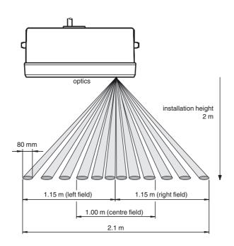
The ProScan is a 12-beam energetic light scanner based on the principles of active infrared. The beams, which are switched independently, enable the sensor to fan out across an extremely wide and narrow detection field in the area of the door.
