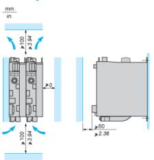
LXM32•U45M2, •U90M2 and LXM32•U60N4 servo drives are cooled by natural convection. LXM32•D18M2, •D30M2, LXM32 •D12N4, •D18N4, •D30N4 and •D72N4servo drives have an integrated fan.
