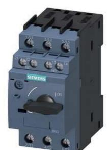
Circuit breaker size S00 for motor protection, CLASS 10 A-release 7...10 A N release 130 A screw terminal Standard switching capacity with transverse auxiliary switches 1 NO+1 NC Reusable packaging Pack = 43 units
