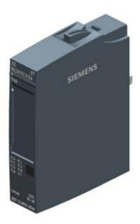
SIMATIC ET 200SP, Digital output module, DQ 8x 24V DC/0,5A Standard, Source output (PNP,P-switching) Packing unit: 10 pieces, fits to BU-type A0, Colour Code CC02, aubstitute value output, module diagnostics for: short-circuit to L+ and ground, wire break, supply voltage
