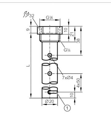
1 fixing bracket for centring piece
