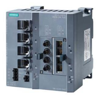
SCALANCE X308-2M PoE; managed IE switch, compact; 4x 10/100/1000 Mbit/s for RJ45 ports electrical with PoE; 2x 100/1000 Mbit/s for 2-port media modules, electrical or optical; LED diagnostics, error signaling Contact with select/set button, PROFINET IO device, network management, Integrated redundancy manager, office features (RSTP, VLAN, IGMP,...) C-plug in scope of delivery
