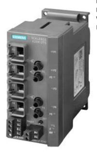
SCALANCE X204-2TS; MANAGED IE SWITCH; 4 X 10/100MBIT/S RJ45 PORTS; 2 X 100MBIT/S MULTIMODE BFOC; LED-DIAGNOSIS; FAULT SIGNAL- CONTACT WITH SET BUTTON; REDUNDANTE POWER SUPPLY; PROFINET-IO DEVICE; NET WORK- MANAGEMENT; INTEGR. REDUNDANCY MANAGER; INCL. ELECTRON. MANUAL ON CD; C-PLUG OPTIONAL
