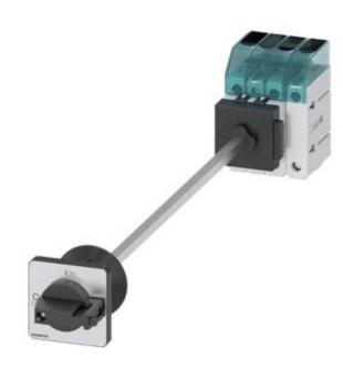
Switch disconnector 3LD3, main switch 3-polig + N, lu 40A operational switch at AC-23 A at 400 V 15,0 kW floor mounting Base mounting with door coupling center-hole 22,5 mm knob-operated mechanism black 48 x 48 mm
