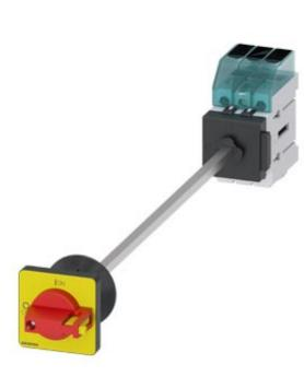
Switch disconnector 3LD3, main switch 3-polig, lu 40A operational switch at AC-23 A at 400 V 15,0 kW floor mounting Base mounting with door coupling center-hole 22,5 mm knob-operated mechanism red/yellow 48 x 48 mm
