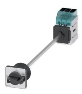
Switch disconnector 3LD3, main switch 3-polig, lu 40A operational switch at AC-23 A at 400 V 15,0 kW floor mounting Base mounting with door coupling center-hole 22,5 mm knob-operated mechanism black  $48 \times 48 \text{ mm}$
