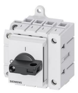
Switch disconnector 3LD3, main switch 3-polig + N, lu 40A operational switch at AC-23 A at 400 V 15,0 kW Distribution board mounting Base mounting with knob-operated mechanism black with auxiliary 1NO+1NC
