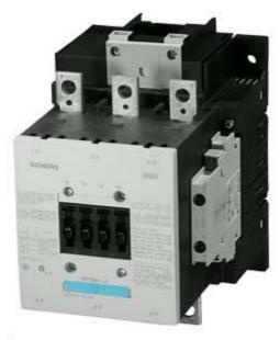
CONTACTOR, 275A/AC-1, AC(40...60HZ)/DC OPERATION UC 220...240V AUXIL. CONTACTS 2NO+2NC 3-POLE, SIZE S6 BAR CONNECTIONS CONVENT. OPERATING MECHANISM REUSABLE PACKAGING 1 PACK = 9 UNITS
