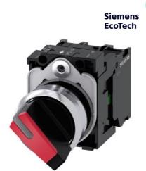
Toggle switch, illuminated, 22 mm, round, metal, shiny, red, knob, short, 2 switch positions O-I, latching, actuating angle 90°, 10:30h/13:30h, with holder, 1 NO, 1 NC, LED red, 24 V AC/DC, screw terminal
