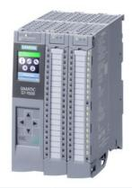
SIMATIC S7-1500 compact CPU CPU 1511C-1 PN, central processing unit with work memory 300 KB for program and 1.5 MB for data, 16 digital inputs, 16 digital outputs, 5 analog inputs, 2 analog outputs, 6 high-speed counters, 4 high-speed outputs for PTO/PWM/frequency output, 1st interface: PROFINET IRT with 2-port switch, 25 ns bit performance, including push-in front connector, SIMATIC Memory Card required
