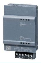
SIPLUS S7-1200 SB 1223 2DI/2DQ based on 6ES7223-0BD30-0XB0 with conformal coating, -20...+60 °C, start up 0 °C, digital input/output 2 DI 24 V DC/2 DQ 24 V DC
