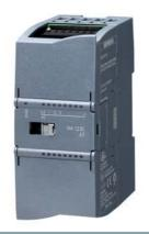
SIPLUS S7-1200 SM 1231 TC based on 6ES7231-5QD32-0XB0 with conformal coating, -20...+60  $^{\circ}\text{C}$  , analog input, 4 AI thermocouples
