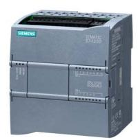
SIPLUS S7-1200 CPU 1212C DC/DC/relay based on 6ES7212-1HE40-0XB0 with conformal coating, -40...+70 °C, start up -25 °C, signal board: 0, compact CPU, DC/DC/relay, onboard I/O: 8 DI 24 V DC; 6 DQ relay 2 A; 2 AI 0-10 V DC, power supply: DC 20.4-28.8 V DC, program/data memory 75 KB
