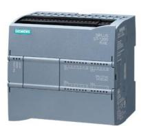
SIPLUS S7-1200 CPU 1214C DC/DC/DC based on 6ES7214-1AG40-0XB0 with conformal coating, -40...+70 °C, start up -25 °C, signal board: 0, compact CPU, DC/DC/DC, onboard I/O: 14 DI 24 V DC 10 DQ 24 V DC 2 AI 0-10 V DC, power supply: DC 20.4-28.8 V DC, program/data memory 100 KB
