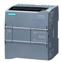
SIPLUS S7-1200 CPU 1212C DC/DC/relay based on 6ES7212-1HE40-0XB0 with conformal coating, -20...+60 °C, compact CPU, DC/DC/relay, onboard I/O: 8 DI 24 V DC 6 DQ relay 2 A 2 AI 0-10 V DC power supply: 20.4-28.8 V D program/data memory 75 KB
