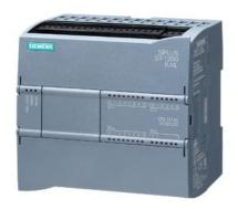
SIPLUS S7-1200 CPU 1214C DC/DC/DC based on 6ES7214-1AG40-0XB0 with conformal coating, -40...+60 °C, start up -25 °C, compact CPU, DC/DC/DC, onboard I/O: 14 DI 24 V DC; 10 DQ 24 V DC; 2 AI 0-10 V DC, power supply: DC 20.4-28.8 V DC, program/data memory 100 KB
