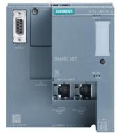
SIPLUS NET IE/PB Link PN IO based on 6GK1411-5AB10 with conformal coating, -40...+60 °C, IE/PB Link PN IO gateway between Industrial Ethernet and PROFIBUS with PROFINET IO functionality S7 routing and data record routing, 10/100 Mbps Fast Ethernet, MRP, 9.6 Kbit/s up to 12 Mbps PROFIBUS, NTP
