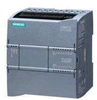
SIPLUS S7-1200 CPU 1212C AC/DC/relay based on 6ES7212-1BE40-0XB0 with conformal coating, -40...+70 °C, start up -25 °C, signal board: 0, compact CPU, AC/DC/relay, onboard I/O: 8 DI 24 V DC; 6 DQ relay 2 A 2 AI 0-10 V DC, power supply: 85-264 V AC at 47-63 Hz, program/data memory 75 KB
